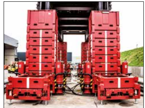
▼ The steel barrels are stacked together to mechanically hold the load.
