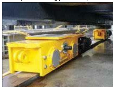
▼ ETR series electric trolley undergoing factory acceptance testing prior to shipment.
